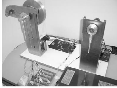
**Figure 2.** Experimental teleoperated system of one degree of freedom.
