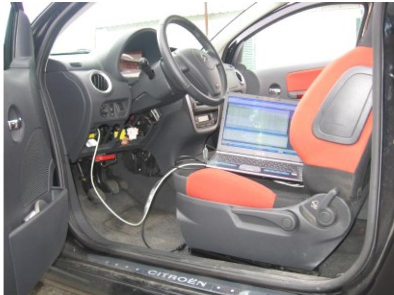
**Figure 7.** Analyzer software tool connected to the OBD connector in a Citroen C2
