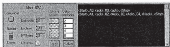
Figura 4: Panel de control del bus I 2 C
